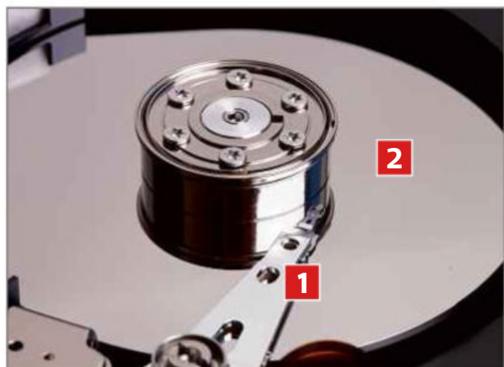
In a hard drive, the magnetic head 1 reads and writes data by moving above the platter 2
